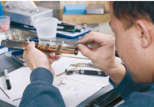
Checking the alignment of the pillars.
