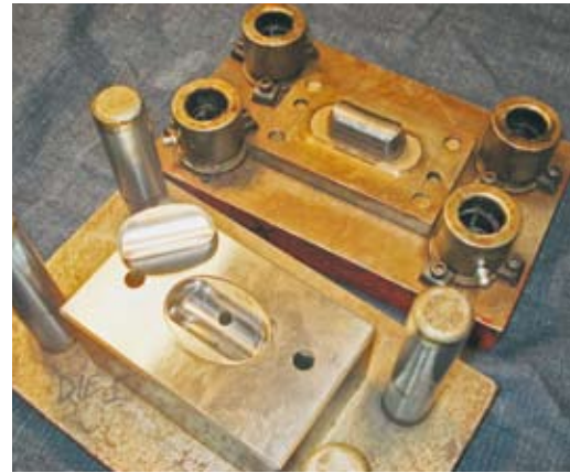
The top and bottom halves of the press tool that stamps out lip-plates.
